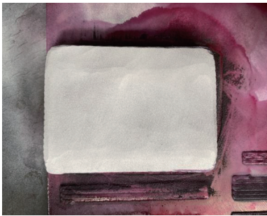
图 4 熔覆块体表面着色探伤 Fig. 4 Surface dye penetrant testing of cladding block
