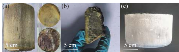
(a)正常原盐; (b)泡沫盐; (c)过滤熔盐
