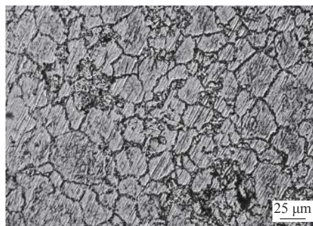
图 1 Ti-10Mo-28Nb-3Zr-6Ta 合金的显微组织 Fig. 1 Microstructure of Ti-10Mo-28Nb-3Zr-6Ta alloy
