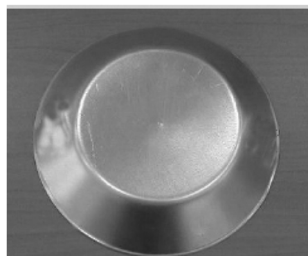
图 2 电磁脉冲成形钛合金试样 Fig. 2 Electromagnetic pulse forming of titanium alloy specimens
